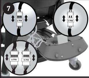
Disconnect the wire harness from the rear module. Remove the old wire harness. Fish through the pass through hole at the bottom of the base. Use caution do not apply tension on the wire harness.
