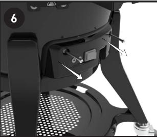
Loosen two screws from rear module.
