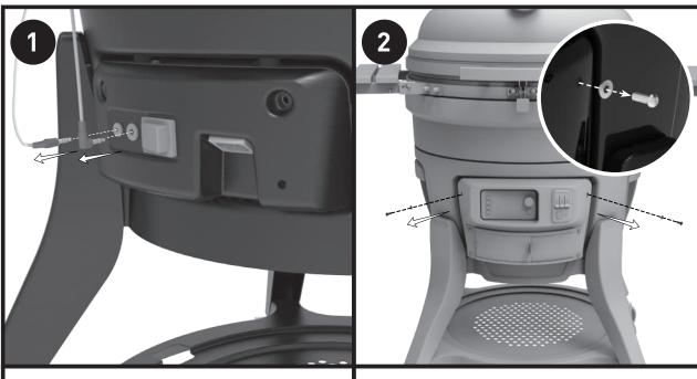
Unplug lid switch, pit probe, and power supply.
