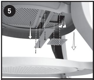
Remove access panels and separate the element from the element plugs.
