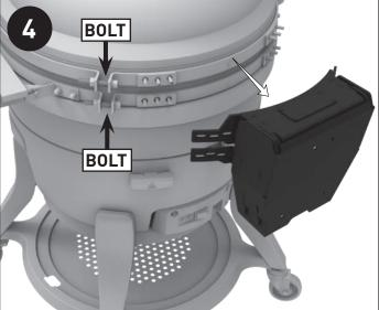
Remove the hinge. Note: You can loosen the bolt on the upper and lower bands if the hinge will not disengage.
