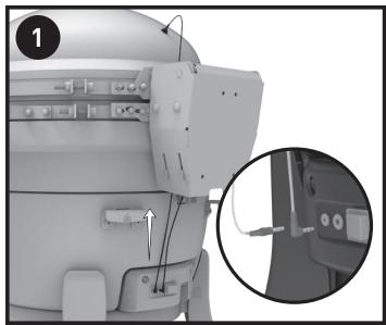
Unplug the pit probe, lid switch, and power supply. from the rear of grill Thread the pit probe and lid switch through the hinge.
