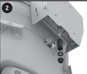
Install the disengagement tool on the hinge.
