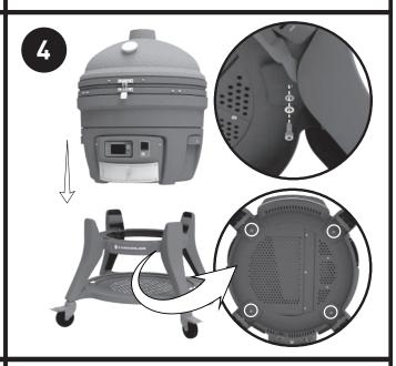
Lower the grill on the cart and secure with 4 screws and washers.
