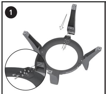
Assemble the legs to top plate.
