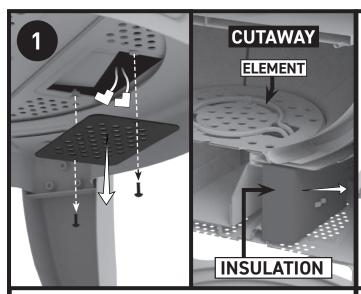
Remove access panel and separate the element from the element plugs. Note: Move the insulation to the side. The insulation should stay inside the grill . It will be reused.
