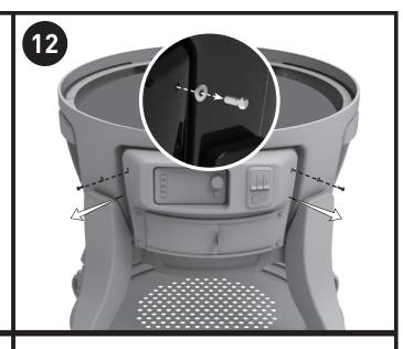
Remove two screws from front module.
