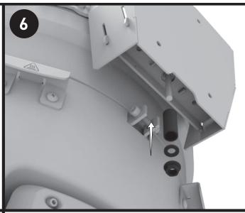
Install the disengagement tool on the hinge.
