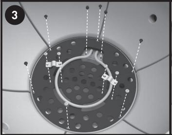
Remove the 2 nuts and 10 screws from the element mounting plate. Remove the 2 brackets.
