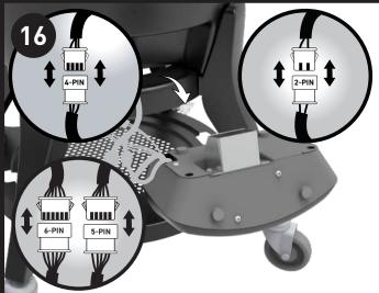
Disconnect the wire harness from the rear module. Use caution do not apply tension on the wire harness. Set the rear module aside, you will need to install this on the new black base kit.
