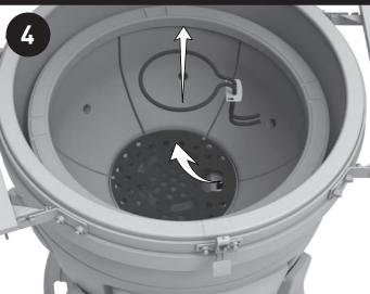
Remove the element from the grill. Note: You will need to turn the element sideways to clear the element mounting plate.
