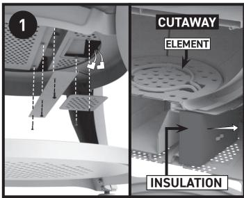
Remove access panels and separate the element from the element plugs. Note: Move the insulation to the side. The insulation should stay inside the grill. It will be reused.
