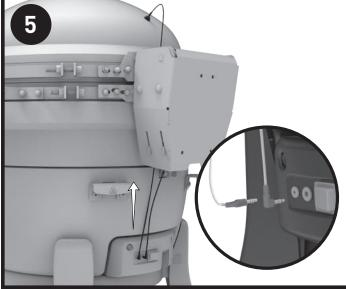
Unplug the pit probe, lid switch, and power supply. from the rear of grill Thread the pit probe and lid switch through the hinge.
