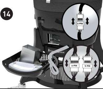
Disconnect the wire harness from the front module. Use caution do not apply tension on the wire harness.
