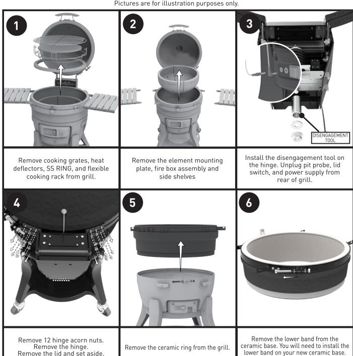
Install the bands and attachments on your new ceramic base. Repeat the steps in reverse order to install the new ceramic base kit.
