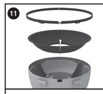
Remove the lower band and stainless steel fire bowl.
