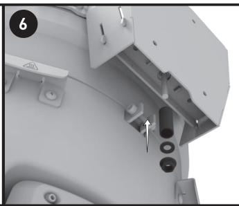
Install the disengagement tool on the hinge.
