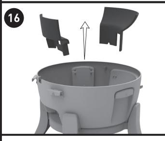
Remove the front and rear insulation.
